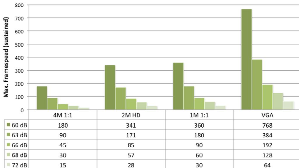
Figure 2. Frame Speed of the Adimec Q-4A180 for various noise improvement scenarios
