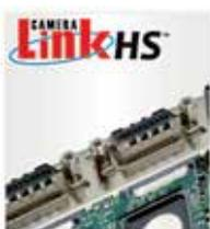
**Camera Link:** Industry default choice for higher speed connectivity where limited cable length and high cable costs are acceptable.
